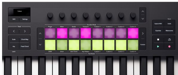
The Launchkey 25 pads reflecting the mixer Mute and Solo states on the pads.
