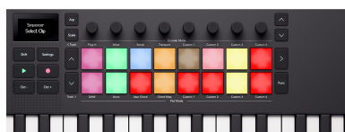
The Launchkey's pads showing the clips you can select. Empty clip slots light red.
