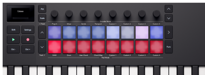
The Launchkey Mini 25 pads reflecting the track select and record arm states on the pads.
