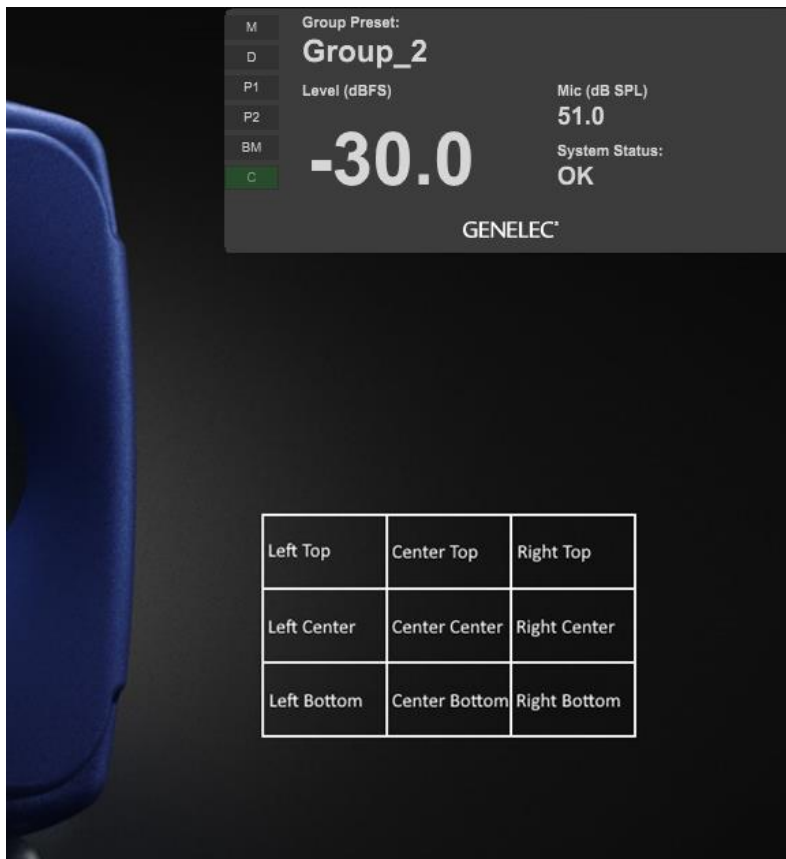
Figure 44. GLM Level Panel.
